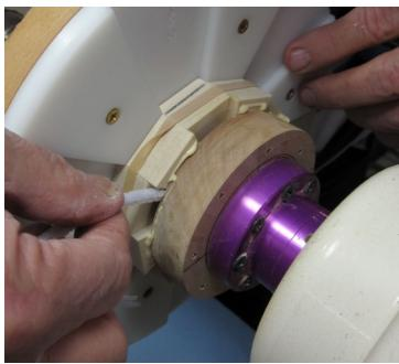
With a dampened — not wet — pipe-cleaner, clean out the excess glue.
