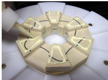
Using the tailstock, apply just enough pressure to set the glue.
