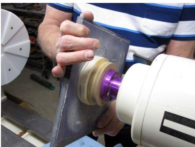
I use a piece of PVC plastic with a sheet of 80-grit sandpaper attached, to flatten the ring. The advantage of this process is that no expensive drum sander is required.
