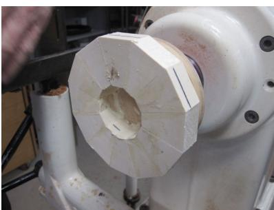
Remove any excess glue from the center of the ring.
