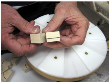
Half of the segments cut with the Wedgie Sled are marked inside, and half outside.
