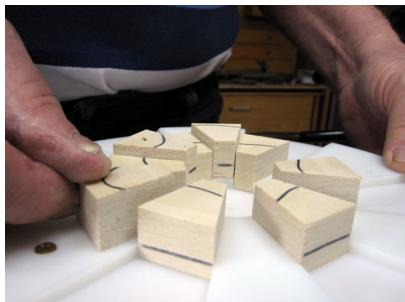
Intersperse the remaining segments marked on the inside, on top of the plate ribs snugly in between the segments in the grooves.
