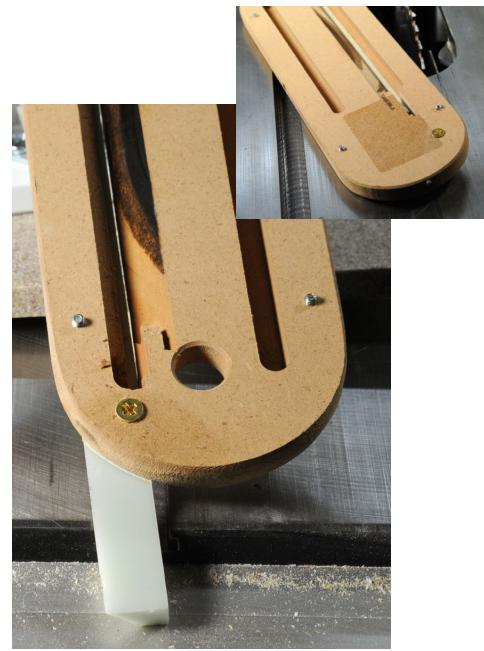
Drill, tap and countersink holes for a 10-24 machine screw through the insert and ramp strip. Do this on both ends. The ramp strip must not protrude above the sled. If it does, sand down until level or slightly below.
