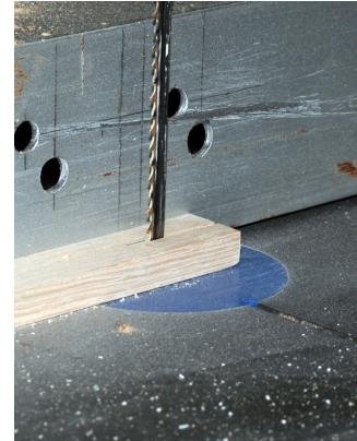
**Cut** a slot down the center of the slide about 1-1/2 inches long.
