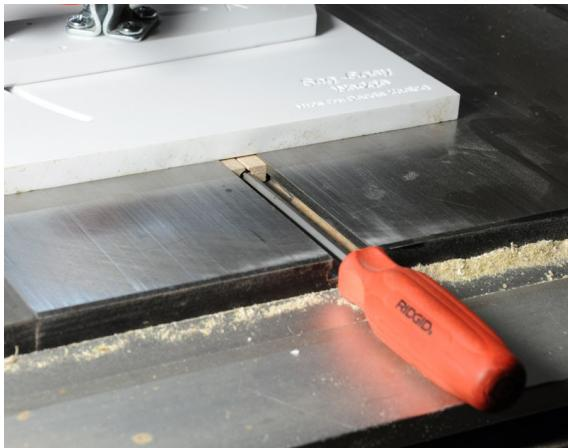
**Crank** the saw blade all of the way down and put the sled in place.
