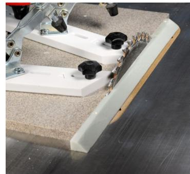
The ramp encourages the segments to fall away from the blade. They can pile up and encroach on the blade. Before this happens, **stop the saw** and move them out of the way. This picture is without the blade guard. I never cut segments without the guard.
