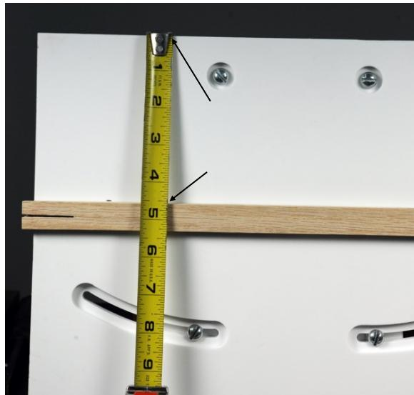
**Transfer** this measurement to the Wedgie sled. This allows a saw blade's width for trimming of the sled.
