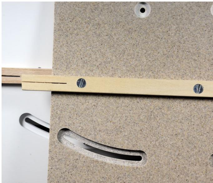
**Add** Anti-friction UHMW tape to the sled.
