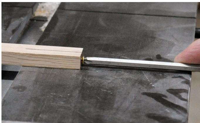
**Install** a no 4 brass wood screw flush with the end of the strip. It will be adjusted later to correctly fit in the saw slot.
