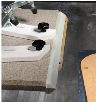
With the Wedgie sled in place as shown, stick down the ramp strip to an MDF plate saw insert. Make sure the strip is against the sled.
