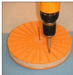
For the required stiffness, attach the SegEasy plate to two 3/4" thick pieces of MDF or plywood cut to the same diameter as the plate, using #6 x 3/4" flat-head wood screws. Drill a 1/8" center hole through the MDF disk. This hole must be absolutely perpendicular or alignment errors can occur when gluing the segments. Use the drill bit as a pin to align the SegEasy Plate with the MDF. Drill the holes for the #6 x 3/4" flat-head screws with a self-centering bit and attach.
